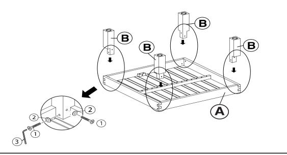
Place the Table Top (A) with its underside skywards onto a clean, soft surface to avoid any scratch or damage to the product.
