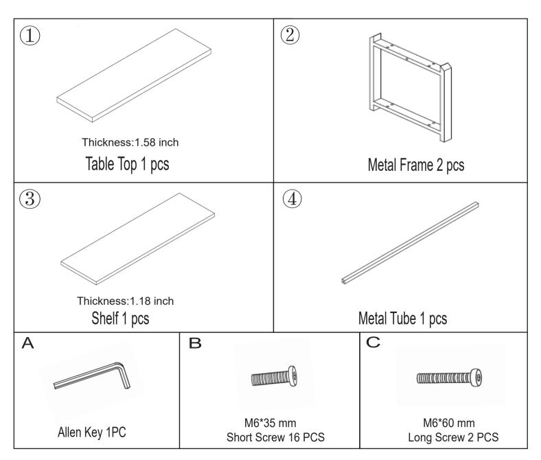
Lay the Metal Frames(2) Parallel to each other on a clean smooth surface such as carpet or cardboard.Fasten Metal Legs(2) to the Metal Tube(4) by using two Long Screws(C) with Allen Key(A).
