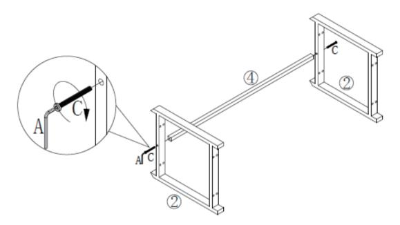
Step 02 NOTE: If holes don't align, loosen all bolts and adjust the holes slightly. After all holes are aligned, fully tighten all bolts.
