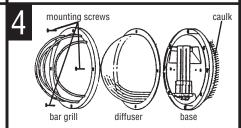
PLACE DIFFUSER ON FIXTURE BASE. Then place bar grill or frame over diffuser and attach to base with mounting screws (8-32 x 1/2, 4 combination head screws provided). NOTE: Outdoor wall fixture MUST be caulked with an acrylic caulk where base of fixture meets mounting surface. This provides a water tight seal when fixture is installed.
