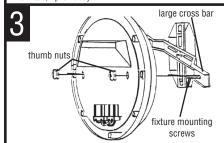
POSITION THE FIXTURE over large cross bar and secure in place with thumb nuts (2 provided). Insert compact type lamps rated 9 watts into sockets. Be sure to use compact type lamps with wattage no greater than specified for this fixture.
