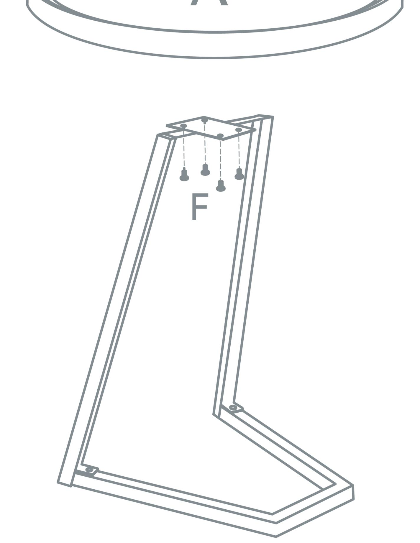
Using Screws (F) fasten the Table Top (A) to the Mounting Plate (D).
