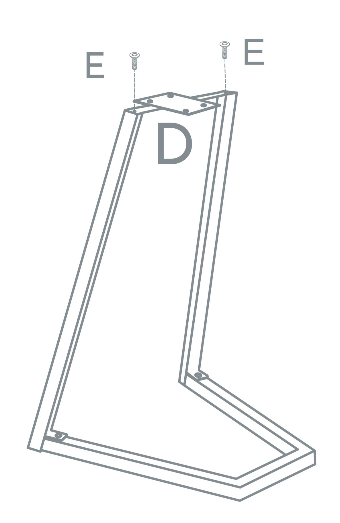
Using Screws (E) fasten the Mounting Plate (D) to the Legs (B).
