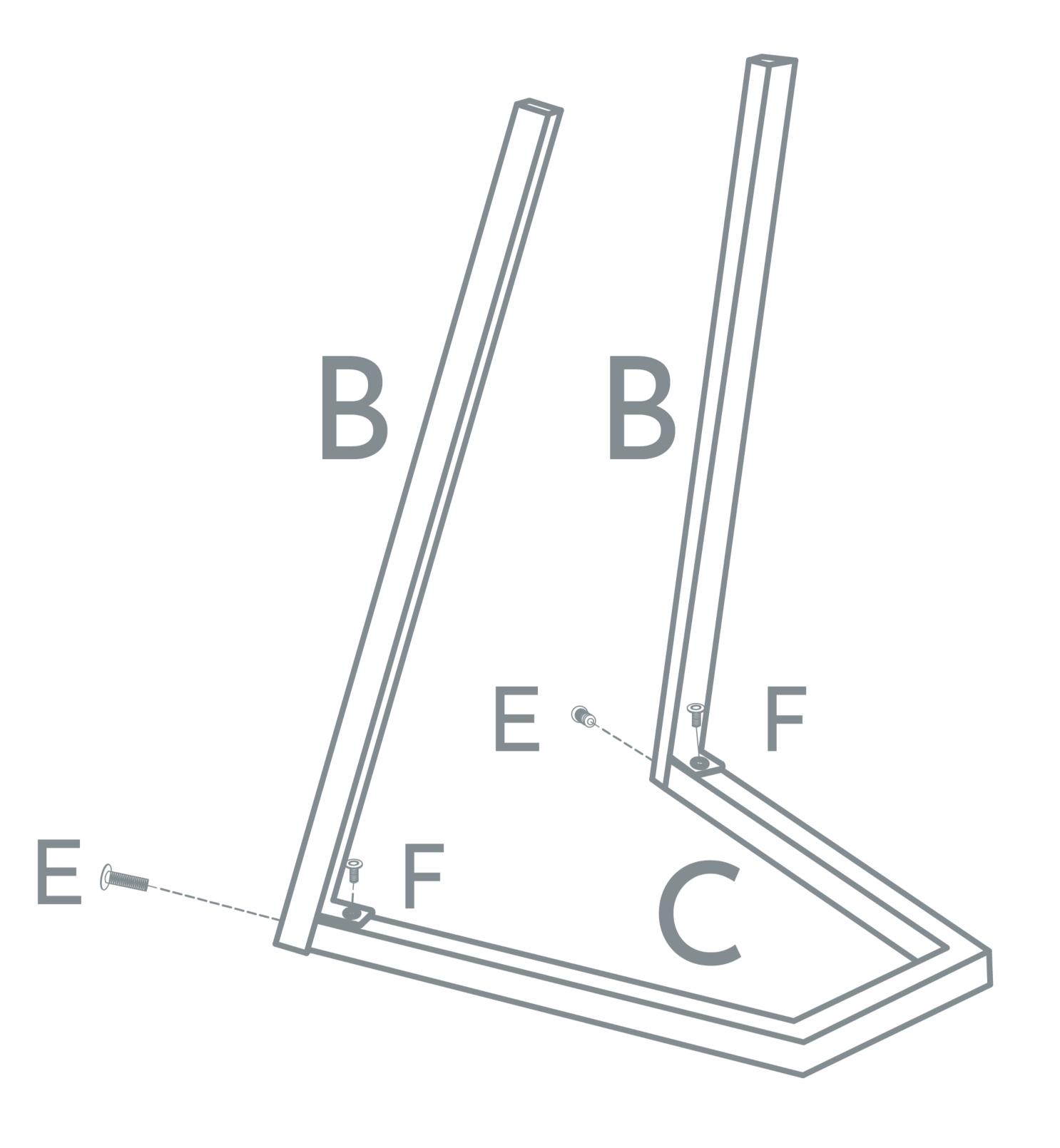
Use Hex Key (H) and Screws (E and F) to fasten the Base (C) to the Legs (B).
