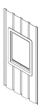
The window set is only used to replace YX- Series metal shed with 156x43cm metal wall panels
