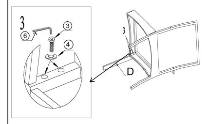
Place the Left Armrest / Leg(D), as picture above so as to be attached to the Left Armrest / Leg(D) and Seat(B) using Hardware (3 4) with Allen Key(6) as shown in Picture3. **Do not fully tighten the bolts.**
