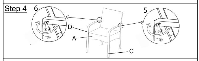
Connect the Armrest/Leg (C&D) to Backrest (A) using Hardware(1) 4) with Allen Key (6) as shown in Picture 5 and Picture 6
