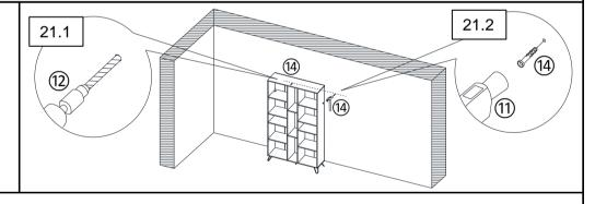
**21.1)** Drill two holes on wall at same height as Metal Brackets((13)) on Multi-Functional Cabinet with Power Drill((12)).
