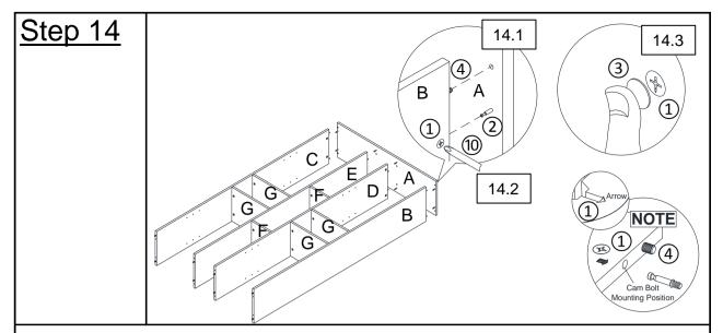
**14.1)** Insert Positioning Dowels(④) on Left Side Panel(B), Left Center Panel(D), Right Center Panel(E) and Right Side Panel(C) into Top Panel(A).
