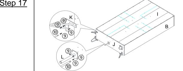
Attach Legs(K) and Middle Leg(L) to Bottom Panel(J) using Screws(9) with Screwdriver(10).
