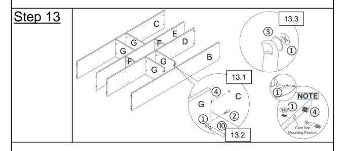
**13.1)** Insert Positioning Dowels(④) on Big Middle Panels(G) into Left Side Panel(B).
