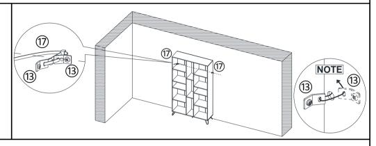
Move the Multi-Functional Cabinet back against wall. Pull the Restraint Straps( $\mathfrak{T}$ ) through the Metal Brackets( $\mathfrak{T}$ ) on the wall and Multi-Functional Cabinet one by one, and pull the Restraint Straps( $\mathfrak{T}$ ) tight.
