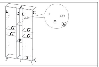
Insert Metal Shelf Support(⑥) into mounting positions on Left Side Panel(B), Right Side Panel(C), Left Center Panel(D) and Right Center Panel(E) by hand.
