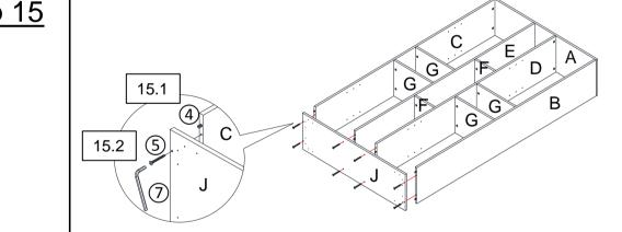
**15.1)** Insert Positioning Dowels(④) from Left Side Panel(B), Right Side Panel(C), Left Center Panel(D) and Right Center Panel(E) into mounting positions on Bottom Panel(J).
