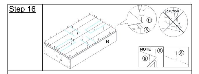
Attach Back Panel(I) to Multi-Functional Cabinet Assembly using Nails(®) with Hammer((11)).
