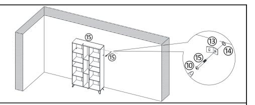
Attach Metal Brackets(13) to Wall Plugs(14) using Wall Plug Screws(15) with Screwdriver(11).
