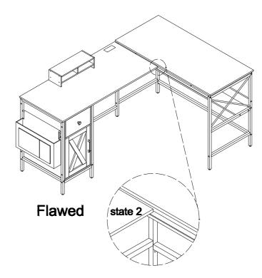
If you encounter "state 2" during the installation process, please loosen the corresponding screws of each part in time, adjust slowly, and then slowly tighten all the screws after the adjustment is completed.
