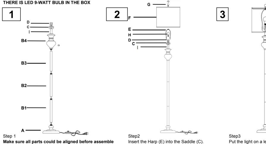
Do not rotate lamp body too hard avoid base screw broken Put the shade(F) on the Harp(E), then
