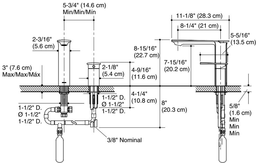
**NOTE:** To simplify future servicing, install an access panel to reach the plumbing.
