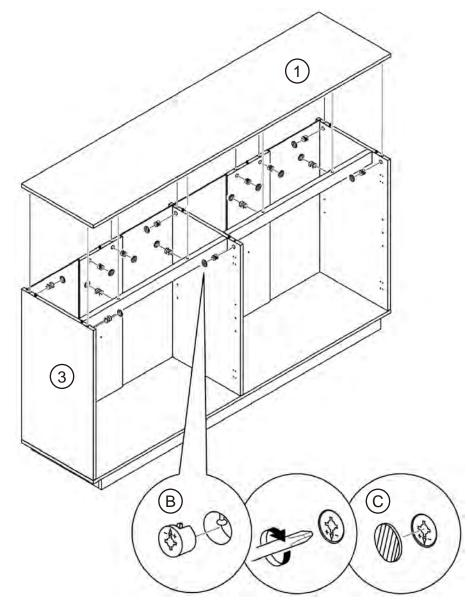
Secure all the back panels in place. 14 16x J Ø3 x 17 16x K K J
