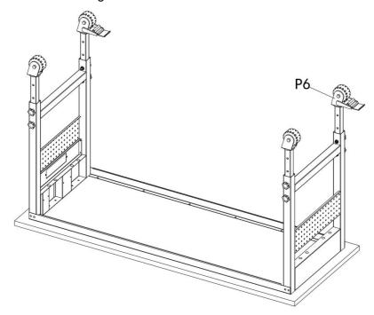
5. Tighten all bolts and nuts, reverse the workbench. As the below picture, using M4X12 screw to fix P11 to P3.
