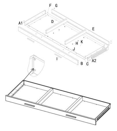
7. Tighten all screws and nuts, install the drawer to workbench, then Finish.For workbench with drawer, the side board and rail were pre-installed at the production factory
