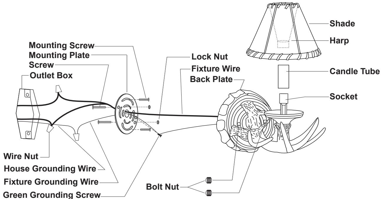
1. Thread two screws to the mounting plate, and secure them with two lock nuts. Adjust the length of the screws if necessary.
