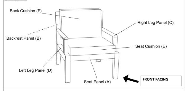
This Chair has multiple parts and may require up to some 30 minutes to assemble. To give you an overview of the Chair parts, the above picture is to help you put the various parts into perspective. Please read through the instructions below to familiarise youself with the parts and steps before assembly.
