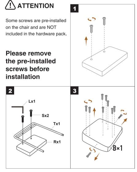
**Note:** All screws havebeenpreassembled to the accessories Please remove them from the accessories before assembling
