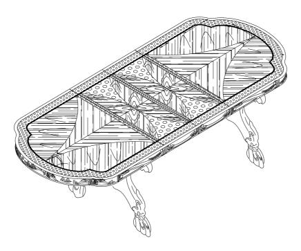
Step 4&5: Flip table right side up (use 2 people)—open table top—you may need to unlock the latches under the top. Place leafs into place lining up and insertin pins into the top, then push close.
