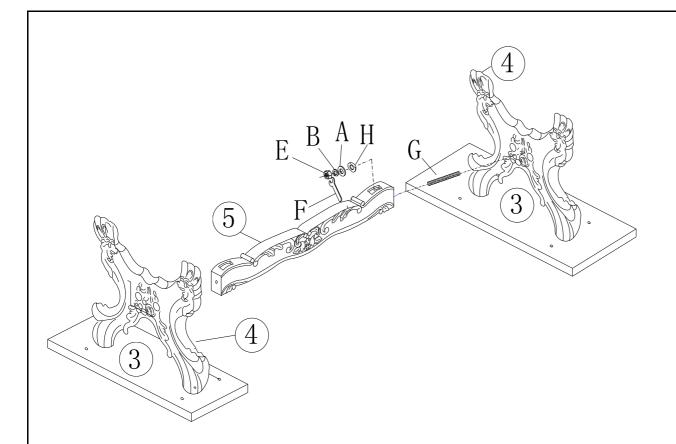
Step 2: Put base upside down on soft non adrasive surface. Assembly stretcher, using #G bolts insert base. Inser #H bolts, #A flat washer, #B lock washer into center hole of seat frame — only hand tighten.
