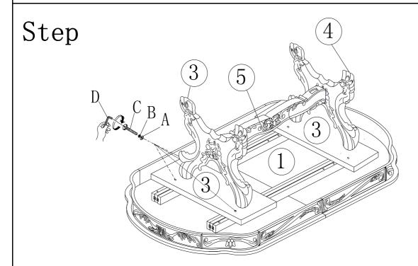
Stpe 3: Put table top spside down on soft non abrasive surface(using 2 people). Turn over bases with mounting plates and place on table runners as shown. Fasten with bolts, lock washer and flat washer. Be sure bolts are tighten with wrench.
