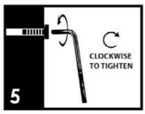
Finally, make sure all parts are properly aligned then use the included **hex key** to completely tighten the screws. Your furniture is now ready for use.
