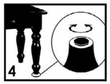
Some furniture come with optional height adjustment knobs underneath each leg. Turn counter-clockwise or clockwise to raise and lower each leg.
