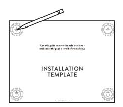
Drill into the wall at each marked location. Use a 1/4" drill bit for brick or other masonry wall. Use a 1/16" drill bit for wood wall.
