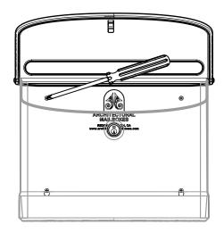
While the mailbox is hanging on the bottom screws, insert the remaining two screws into the top holes and secure with a screwdriver.
