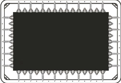
The diagram shows the mat in the frame. More middle springs are now connected to the mat, filling in the gaps between the previously connected ones.
