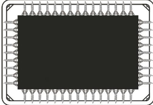
The diagram shows the mat in the frame. All middle springs along all four sides are now connected to the mat, completing the assembly.
