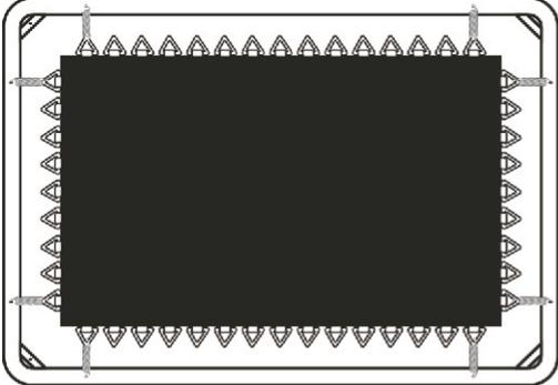
The diagram shows a rectangular trampoline mat (black) placed inside a square frame. The mat is slightly offset from the center. The four corner springs of the frame are connected to the mat. The other springs are not yet connected.
