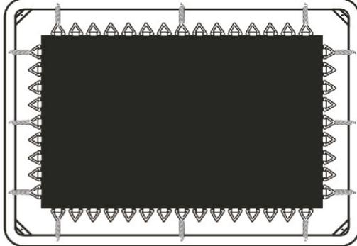
The diagram shows the mat in the frame. In addition to the corner springs, the middle springs along all four sides of the frame are now connected to the mat.
