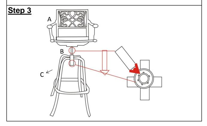
Attach the Chair Seat(A) with attached Iron Plate to the Chair Leg Base(C) as pictured above.
