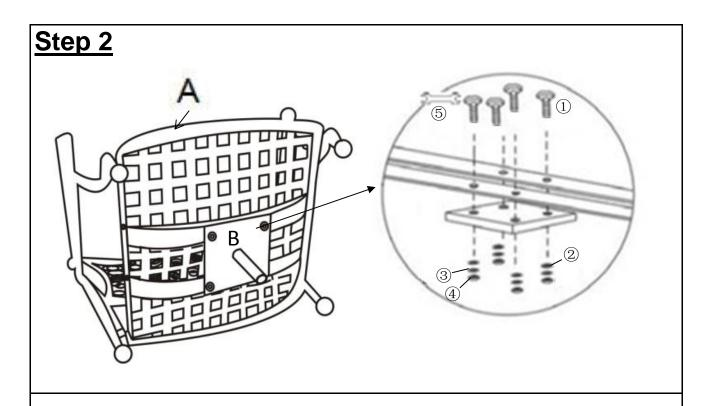
Attach the Iron Plate(B) to the undersidebase of the Chair Seat(A).
