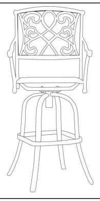
Make sure that the Chair Seat and the Chair Leg Base is fully and firmly attached together as one complete piece
