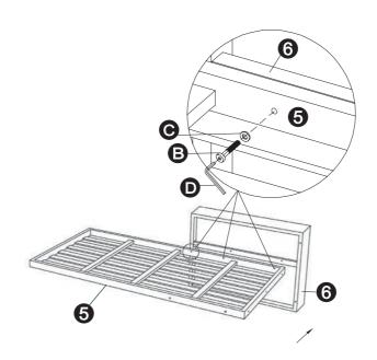
**6.** Attach Support Leg (7) to Seat Panel (5) by using M6X20mm bolt (A) and M6X40mm bolt (B) with Washer (C), and fasten all bolts with Allen Wrench (D).
