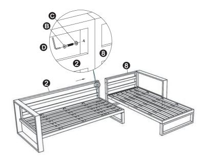
Attach Seat Panel (5) to Seat Panel (1) by using M6X40mm bolt (B) with Washer (C), and fasten with Allen Wrench (D).
