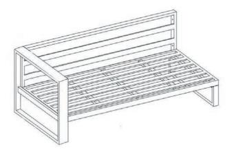
Attach Seat Parts (5) to Side Panel (6) by using M6X40mm bolt (B) with bolt Washer (C), and fasten with Allen Wrench (D).
