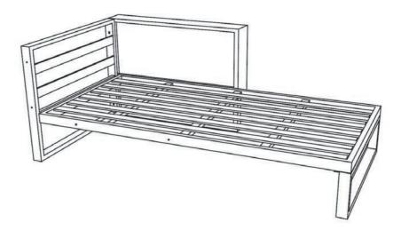
**9.** Attach Back Panel (2) to Back Panel (8) by using M6X40mm bolt (B) with Washer (C), and fasten with Allen Wrench (D).
