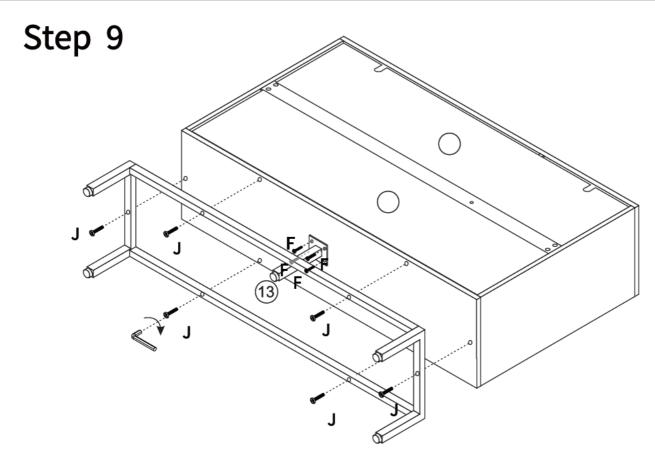
Install the bottom frame to the cabinet by screw (J). Install the middle leg to the cabinet by screw (F) the installation is as shown above.
