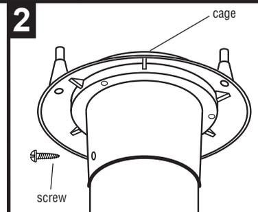
Position the fixture over the post as shown. Fasten with screw at hole in post collar by drilling hole at same location through post and securing with screw.
