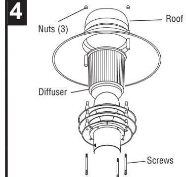
Place diffuser in base and attach roof with screws and nuts.
