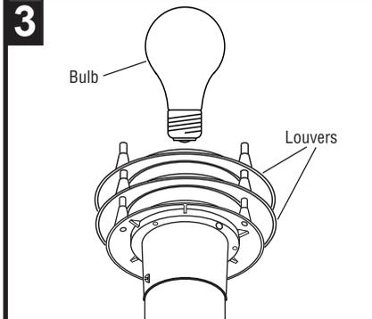
Position louvers to base. Install bulb in socket. Be sure to use bulb with wattage no greater than specified for this fixture.
