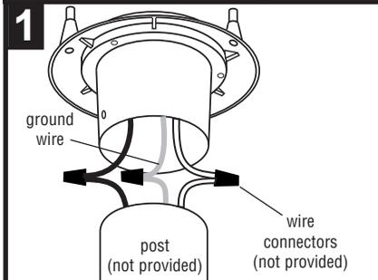
Connect the wires. Note: Attach black fixture wire to black supply wire, white fixture wire to white supply wire. Do not mix them up. Use wire connectors (not provided). Connect bare fixture ground wire to ground from outlet box. NEVER CONNECT GROUND WIRE TO BLACK OR WHITE POWER SUPPLY WIRES.
