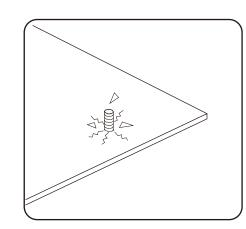
6.Pay attention to avoid cver-tightening fasteners, orthey may induce cracking within the board.
