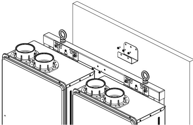
1. Using the holes in the wall hanging bracket, securely attach the bracket level to the wall. Ensure that the attachment strength is sufficient.
