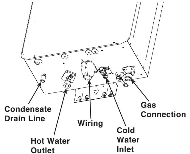
The condensate drain pipe (along its entire length) must be at least the same diameter as the drain line.
