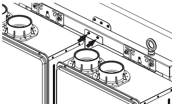
3. Secure the front of the bracket to the front of the wall hanging frame with a #12 x 3/4 drill point screw.
