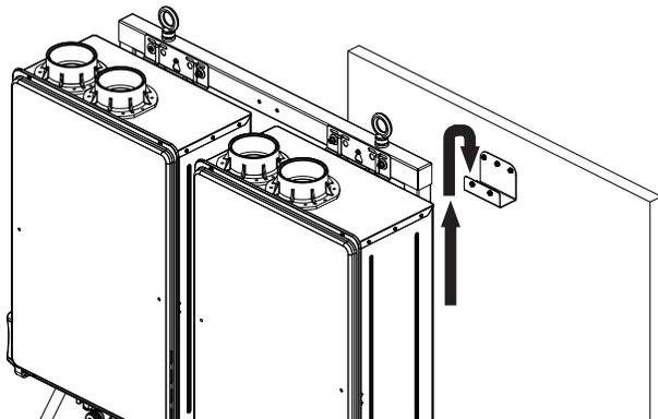
2. Lift the wall hanging rack, and insert the top of the frame into the bracket.
