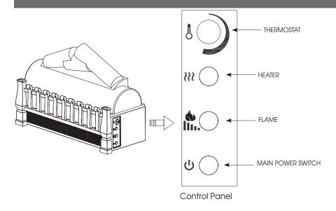
The fireplace can be operated by either the remote control or the control panel.
