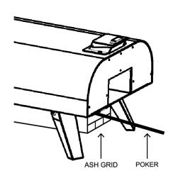
**WARNING:** Pellets may still be warm so heat resistant gloves should be worn when disposing of ash.
