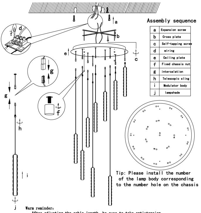
After adjusting the cable length, be sure to take anti-tension treatment, (" 8 "button/lock wire firmware/anti-tension knot, etc.) So as not to cause the safety hazard of the lamp body falling! Finally tear the gray and white protective film on the lamp body.
