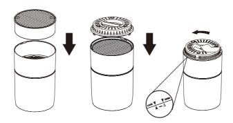
(3) Place the new Composite Filter into the machine, replace the Composite Filter Cover and turn it counterclockwise, from OPEN to LOCK, to secure the Composite Filter Cover to the machine.
