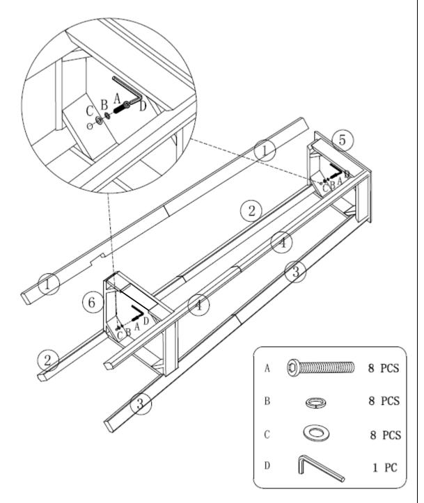
Assemble Posts (1), (2), (3), (4) to Top Panel (5) and Shelf w/Drawer (6) using Bolts (A) with Spring Washers (B) & Flat Washers (C) by Allen Wrench (D).
