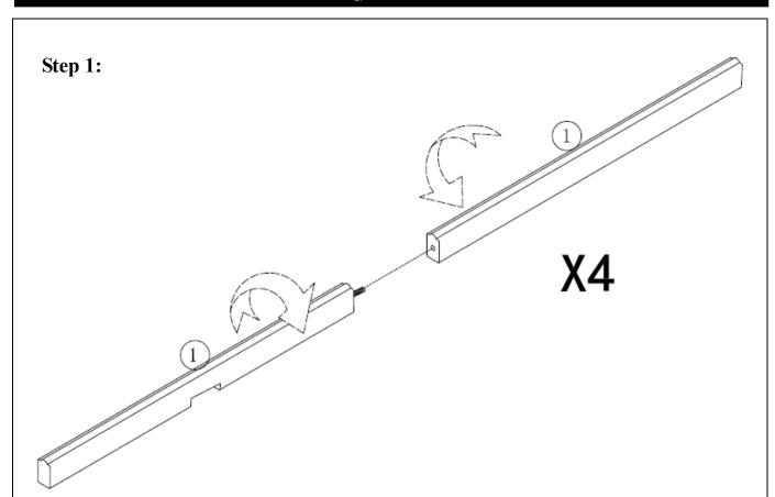
Connect the two Posts (1) together as above shown. Assemble other Posts (2), (3) and (4) in the same way.
