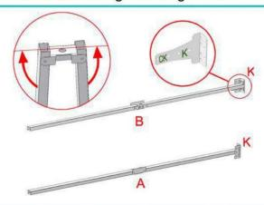
As shown in the figure, extend A and B, and lock K\*2 (headboard bracket) on A and B with L\*4 (small bolt).
