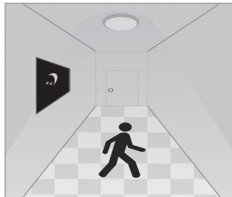
With insufficient daylight, when motion is detected, the light will turn ON.
