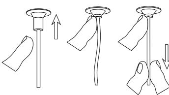
1.Using the tip of your finger or fingernail, depress the pin into the ceiling canopy, this will release the cable locking mechanism
