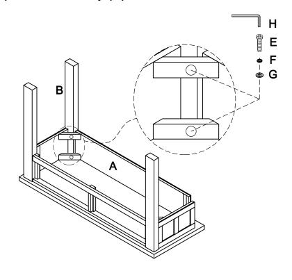
Attach Bottom Panel (C) to the Leg (B) by using Flat Washer (G), Lock Washer (F), Bolt (E) with L-Allen Key (H), and then attach another Leg (B) to the Top Panel (A) and Bottom Panel (C) as below showing.
