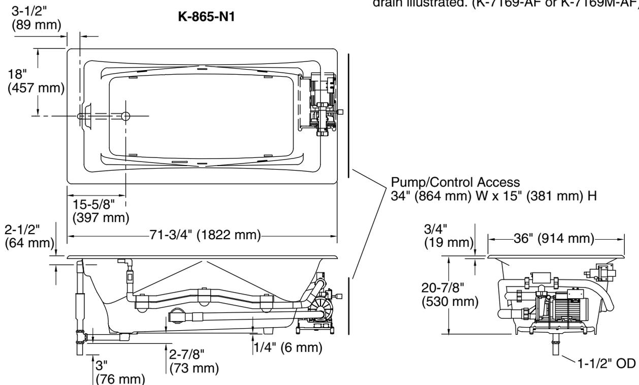
No change in measurements if connected with drain illustrated. (K-7169-AF or K-7169M-AF)
