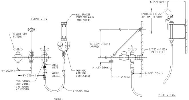
J. INLETS ARE 1/2" NPT FEMALE. ALL DIMENSIONS ARE IN INCHES(MILLIMETER) UNLESS OTHERWISE SPECIFIED AND ARE SUBJECT TO CHANGE WITHOUT NOTICE.
