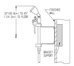
7/09 92-2161-4 Note- The sink fitting does not have to be turned on for the eyewash to operate.
