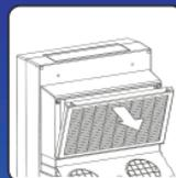
2. Remove the Pre-Filter from the filter frame.
