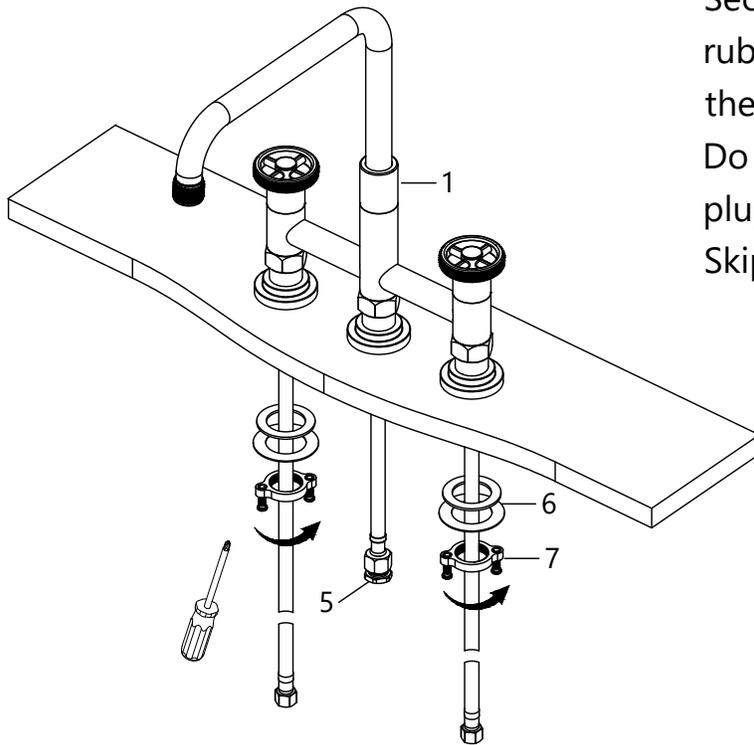
Secure the faucet body (1) with the rubber and metal washers (6) and the mounting nuts and screws (7). Do not overtighten. Make sure the plug (5) is installed tightly. Skip to Step 7.
