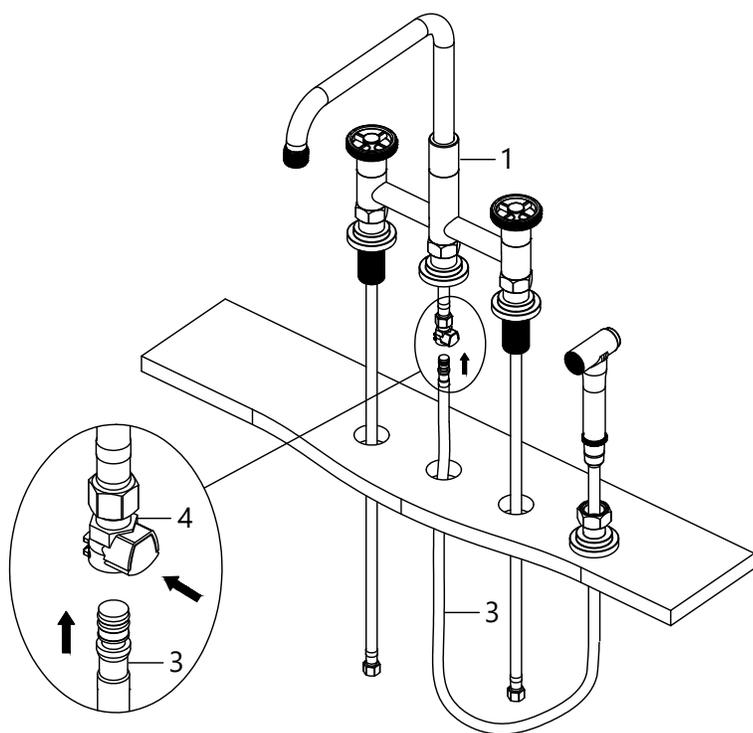
Install the faucet assembly through the holes in the countertop. Remove plug (5) and install quick connector (4). Connect the sprayer hose (3).
