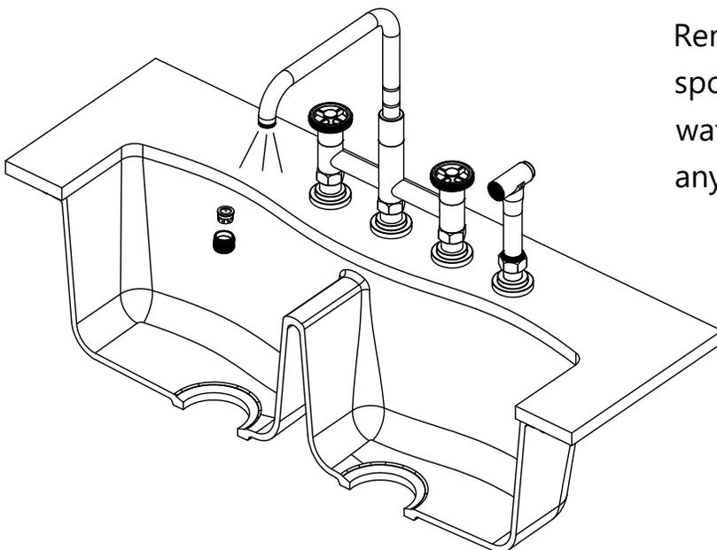
Remove the aerator from the spout. Turn faucet on and let the water run for 60 seconds to flush any debris.
