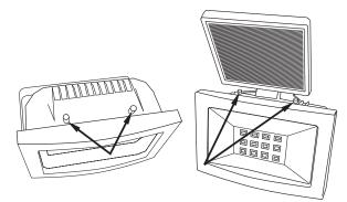
Once you have identified all parts, connect the solar panel to your Solar Powered Flood Light by plugging the 9 foot cord into the cord attached to the bottom of the Solar Flood Light. Firmly turn and twist the cords while pressing together for a tight connection.
