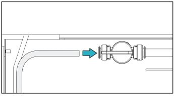
**Note:** Elkay also recommends installing a shutoff valve at the source of the water supply for the water dispenser.
