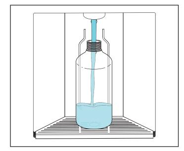
**Note:** The water dispenser is set to automatically shut off after 16 ounces of water has been dispensed to prevent overflow and potential flooding so multiple activations will be required to get the required one gallon of water flow through the unit.
