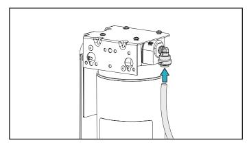
5. Connect the 1/4 inch insulated water line to either a remote chiller or the 1/4 inch water line on the water dispenser. Use a union connection fitting to connect the water line to the water dispenser.
