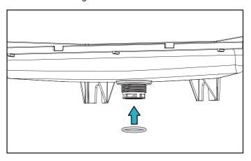
Thread the strainer into the drain adapter.
