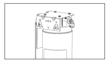
3. Connect a 3/8 inch water supply line, copper or plastic, to the quarter-turn shutoff valve.
