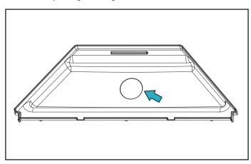
3. Place a small amount of plumbers putty around the lip of the strainer flange and insert it into the hole. If the flange does not fit, carefully open the size of the hole.
