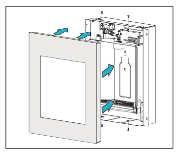
NOTICE It is recommended to attach the front cover with the top two mounting screws to prevent it from falling away from the water dispenser while the filter unit is being installed.
