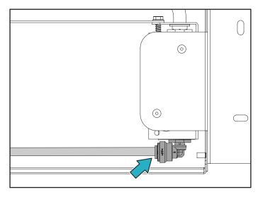
b. If the filter is installed in a remote location, attach an installer supplied length of 1/4 inch tubing to the 1/4 inch tubing from the water dispenser using a union coupling. The type of 1/4 inch tubing, copper or plastic, should meet all local regulations and building codes. This line should be insulated to prevent condensation.
