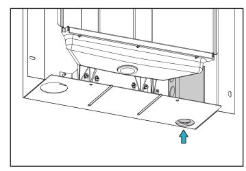
Note: If an optional filter unit will be installed under the water dispenser, the space behind that filter box is limited so make sure any electrical wiring will not interfere with mounting the filter box into the wall. Refer to "4.3 Critical Depth Dimensions" on page 6 for additional information.
