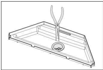
Attach one end of the 3/4 inch flexible drain hose to the 3/4 inch barbed drain adapter connection using the supplied hose clamp. The supplied flexible drain is 13 inches long. If a longer drain hose is required, it must be installer-supplied.
