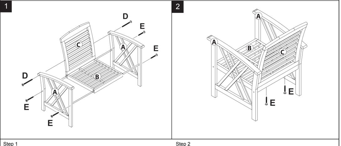
Tighten screw-1 (E) with allen key (H1) to attach back frame(C)
