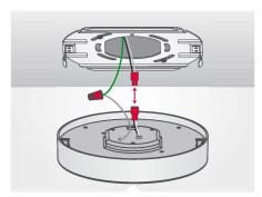
STEP 3: Make ground connection. Next simply "snap" the two sides of the orange wire connector together.
