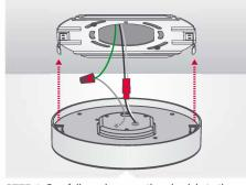
STEP 4: Carefully push connections back in to the J-Box, Align the two clips and driver on the fixture body to the opening of the J-Box Mounting bracket.
