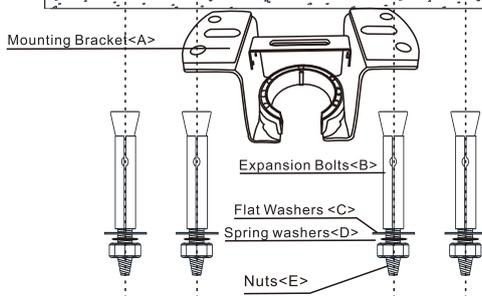
**Note:** According to the ceiling of different materials, use different screws to fix the hanging bracket. Don't fix the hanging bracket on the wood ceiling less than 12MM to prevent danger caused by loosening of screws. After the hanging bracket is completed, ensure that it can withstand the tension test of more than 68KG for safety.
