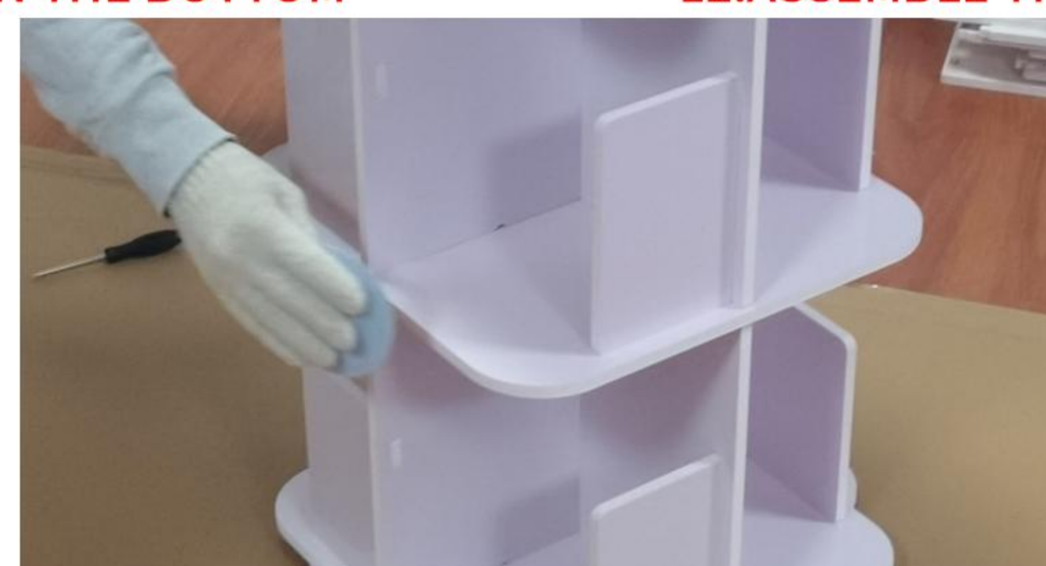
14.IF THE EDGE IS SHARP, YOU CAN USE ABRASIVE PAPER TO POLISH THE EDGE
