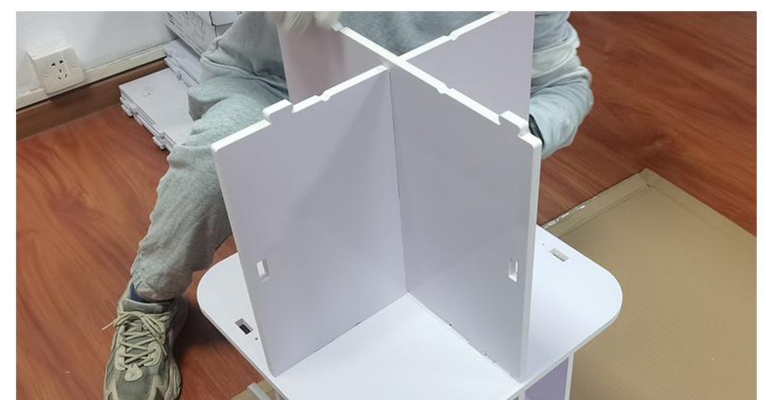
8.ASSEMBLE THE THIRD AND FOURTH B PLATES NOTE: THERE IS A GAP ON THE SIDE OF THE INVERTED ASSEMBLY
