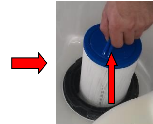
5. Take out the paper filter upwards.
