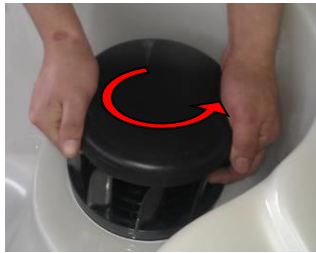
1. Swivel the protection grating anticlockwise.
