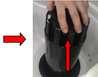
3. Take out the lifting cartridge upwards.
