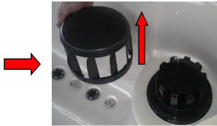
2. Take out the protection grating upwards.
