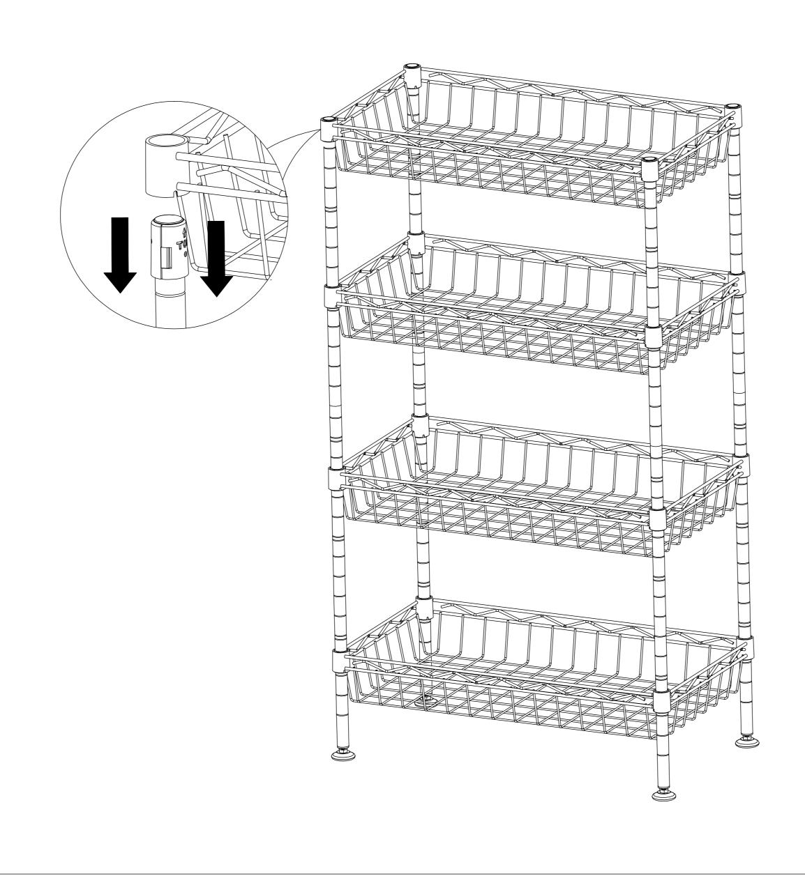
Once all four wire baskets have been installed, pushing firmly down on every shelf at corners by rubber mallet to ensure the shelf in a place over the plastic clips and screw the Leveling Feet in or out to attain proper leveling.
