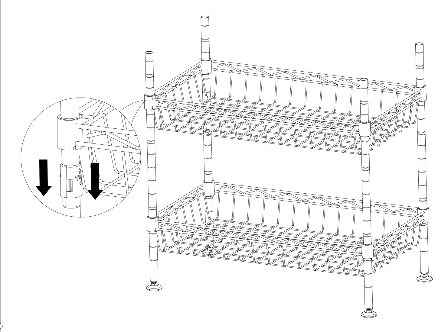
Screw Upper Poles (C) into Lower poles by screw connectors which is already on the upper poles.
