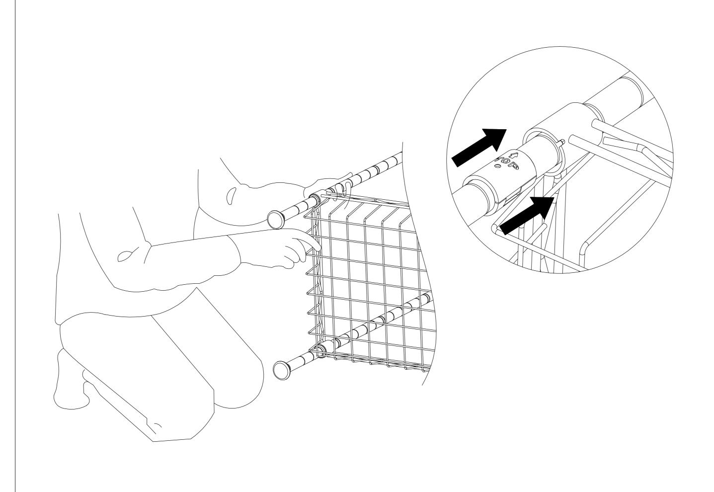
3 Snap Plastic Clips into the pole grooves of the lower poles at your desired basket height position. Slide down the basket from top down onto the plastic clips.
