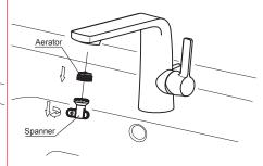
If flow rate of the water gradually decreases after some time, it may results from aerator blockage. Please clean the aerator as shown in figure above: Turn off the handle, disassemble the aerator with the spanner, wash the aerator and then install it back.
