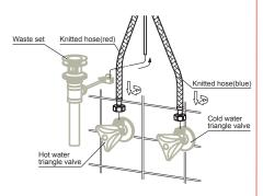
Connect the two knitted hoses to the two triangle valves (Red for hot water and blue for cold water).
