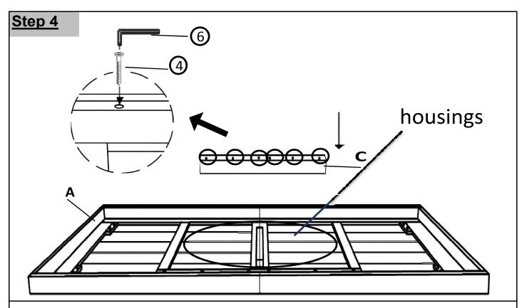
Align Support Bar(C) to the housings on Table Top(A) and secure using Screws(4) with Allen Key(6).
