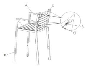
Attach Backrest(D) between Right Leg(B) and Left Leg(A) using Bolts(3) with Allen Key(4) as shown above.
