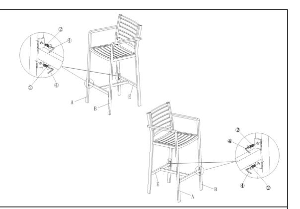
Attach Footrest(E) between Right Leg(B) and Left Leg(A) using Bolts(2) with Allen Key(4) as shown above.
