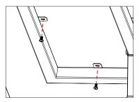
Install screws loosely, do not tighten to allow for adjustment in table alignment.
