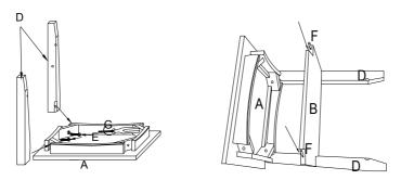
**Step 4** Attach Bottom (C) using 2 Hex Bolts 45mm (E). Repeat same procedure with other 2 Posts (D).
